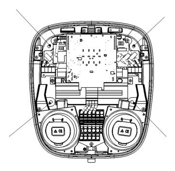
5. Connecting the power cables: Pull the power cables through the slider hatch, approx. 80mm. Strip the cables approximately 20mm. Connect the cables (L1-L3, N & PE) to the WAGO terminals as the picture shows.
