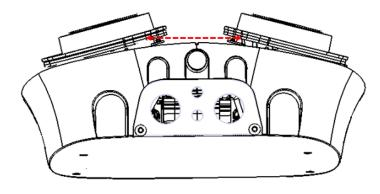
6. If you are going to use ethernet cable, plug it in the RJ45 port on main card as picture shows.
