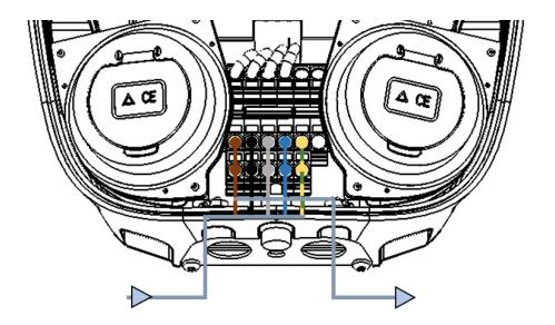
If you are installing Aura on an IT-net. Install the phase cables L1-L3 and install the 1-3 jumper bar, that is included in the kit, according to picture below. L2 and N will be connected.
