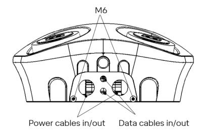
4. Mount Aura on the wall. Use the key to unlock Aura. Rotate the front and unhinge it. Avoid scratching the front when placing it down. Fit Aura on the wall according to the drilled holes. Ensure that the mounting is fixating the Aura firmly.
